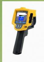
THERMOGRAPHIC INFRARED INSPECTION USED WITH BLOWER DOOR TEST
